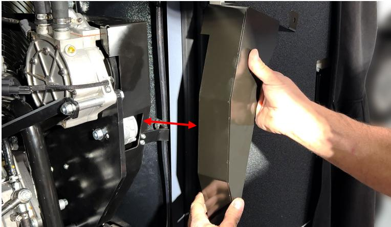
Modify the LHG belt guard assembly (140-0146-A0 for 45kW, 140-0147-A0 for 25kW), using the template in the kit and in Appendix A at the end of this document to cut an opening for the back of the Belt Tensioner.
