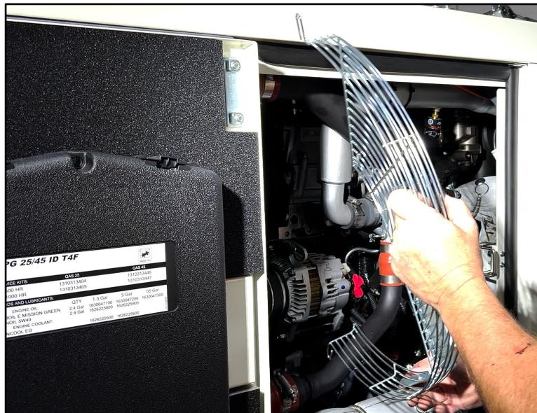
Reinstall fan guard in its stock location using original hardware.
