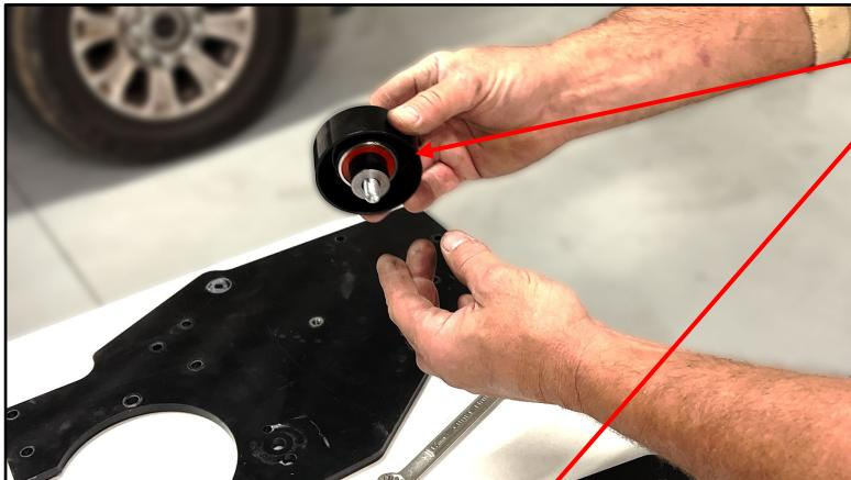
Install the Idler Pulley (981-0005-A0) saved from step 4.8 above, with Idler Pulley Spacer (14-0456-C0) and M10 Washer (925-0031-A0) to the Backing Plate (14-0453-G0), using Hex HD Bolt (920-0019-A0).
