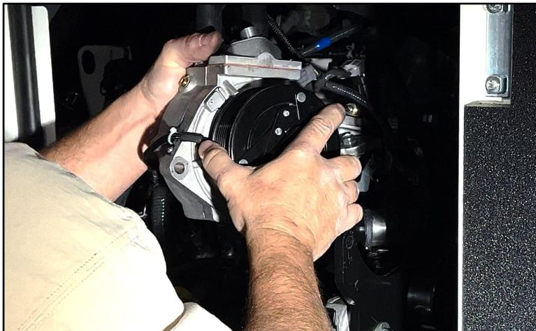
Holding the LHG, remove the right side mounting bolt, spacer, and washers, and carefully set the LHG aside.
