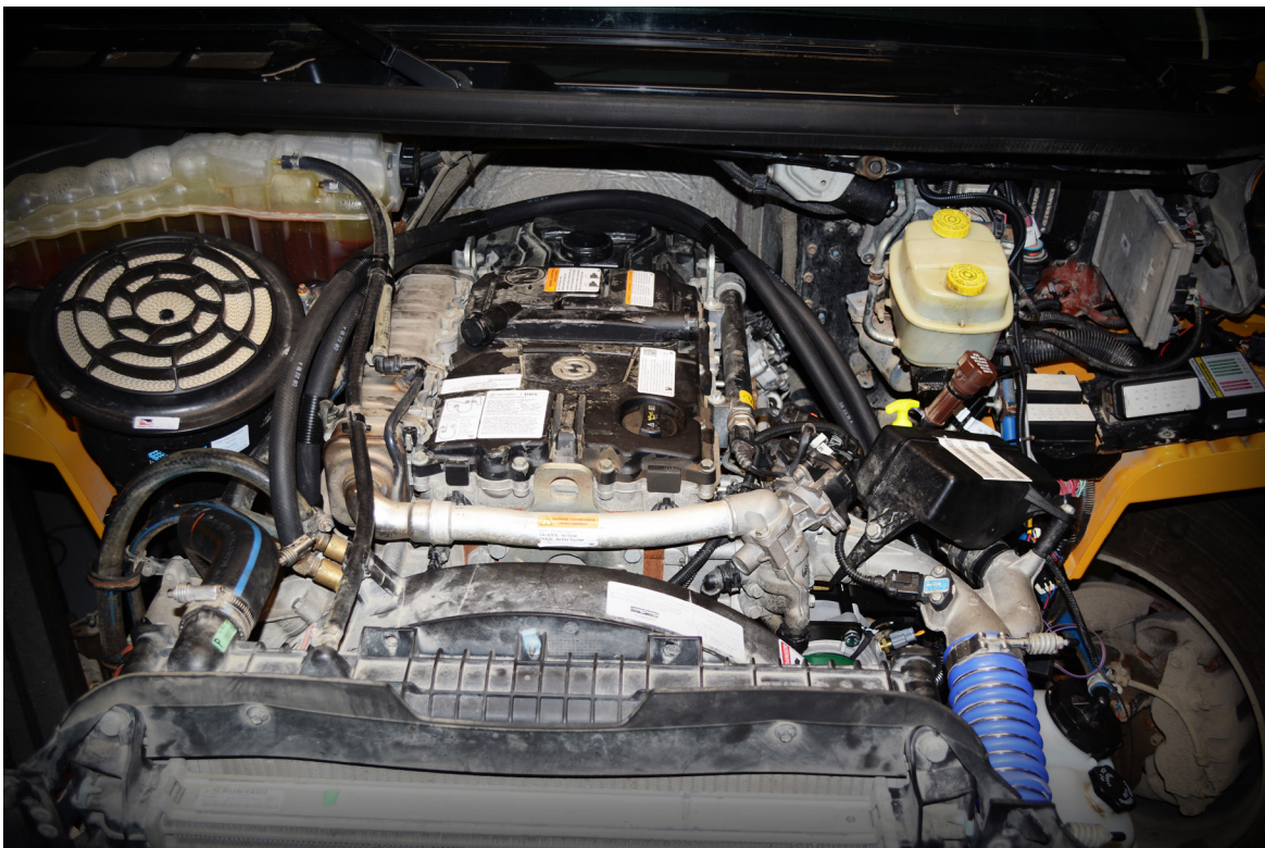
Figure 8 - Aerial View of Installed Hoses
